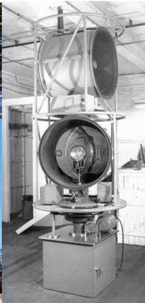
The first 'headlamp' type light in an Australian lighthouse was this one designed and manufactured in Australia in 1962 and installed in the lighthouse at Marino Rocks in South Australia.
