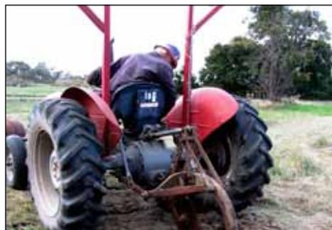
*Rabbit hole ripper attached to Fordson tractor*
