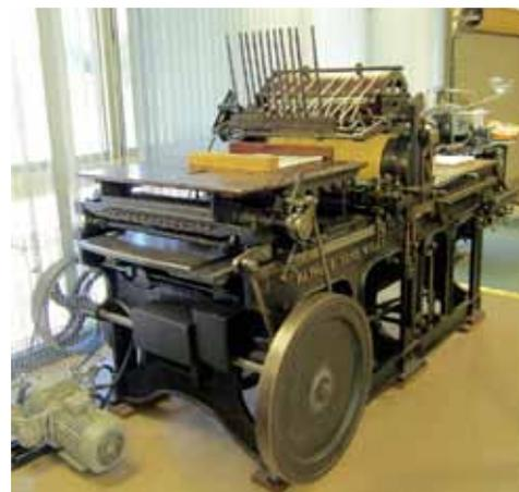
*The Wharfedale printing machine was the "bread and butter" machine of printers for both commercial work and newspaper production. Originally it would have printed between 1,000 and 1,200 papers per hour.*
