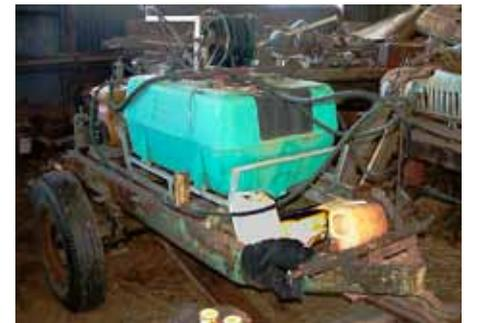
*Spray tank made by Hedley for killing noxious weeds, mounted on a utility chassis*
