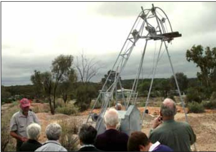
*ASHET party in 2011 viewing an auto-hoist at Lightning Ridge. This simple machine, invented at Lightning Ridge, allows a miner working on his own at the bottom of a shaft, to hoist a bucket of ore to the surface and dump it on the stockpile.*
