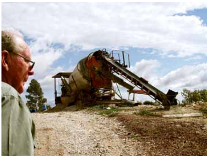
Wet puddling at Lightning Ridge
