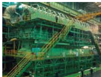
Wärtsilä-Sulzer diesel engine for large container ship
